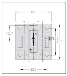
Positioning unit 100 with automatic stopper
