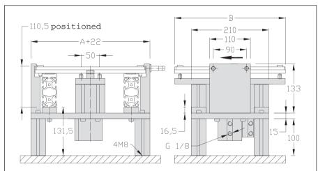
$A = workpiece carrier width \\ B = workpiece carrier length$
