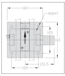
Positioning unit 100 with automatic stopper
