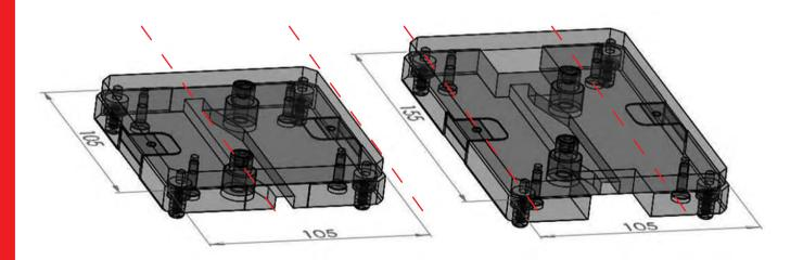
The lay-out of guide pins is identical in width. However, in the length direction, the guide pins of a 105x155 workpiece carrier have a larger gap than the 105x105 workpiece carriers. In case of use of workpiece
