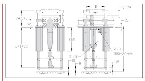
B = workpiece carrier length
