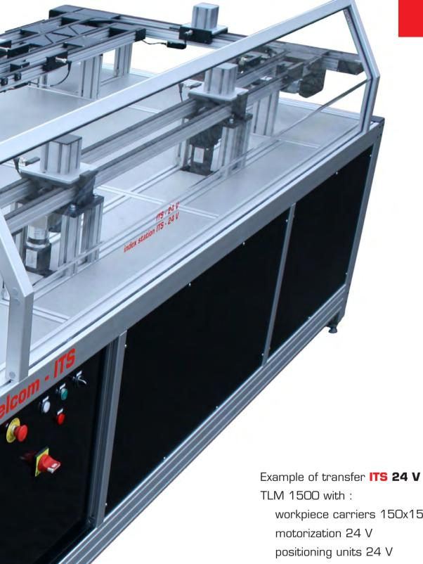
workpiece carriers 150x150 stoppers 24 V
