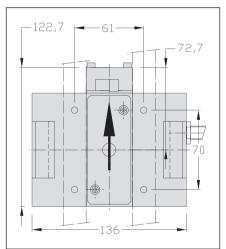
Positioning unit 100 with automatic stopper
