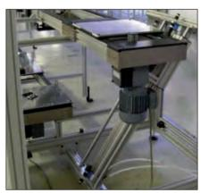
Inclined transfersystem lift-upper or basement type  $% \left( 1\right) =\left( 1\right) \left( 1\right) \left$
