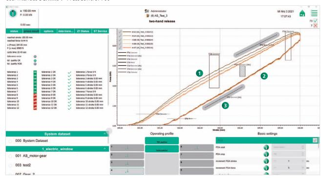
1 + 2 All tolerances can also be used inverted (blocking ranges)
