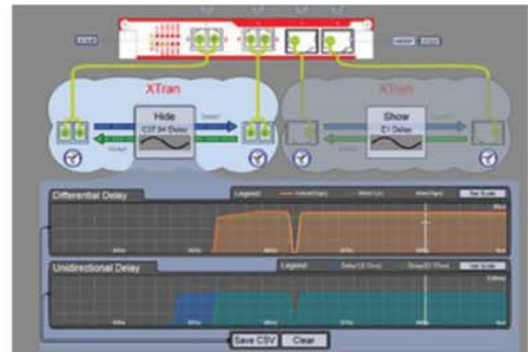
Fig. 4. Asymmetrical (or differential) delay monitoring
