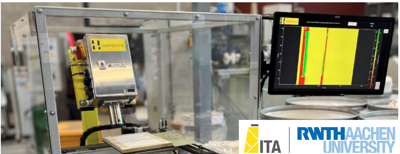
Measurement of surface uniformity of dry-laid paper using the Hammer-IMS laboratory measurement system.
