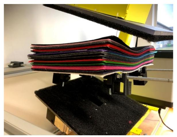
Fig. 2: Picture of an M-Ray weight measurement of a 47 mm thick, 9.6 kg/m<sup>2</sup> stack of various-colored synthetic nonwoven products, placed between the transmit and receive antennas.
