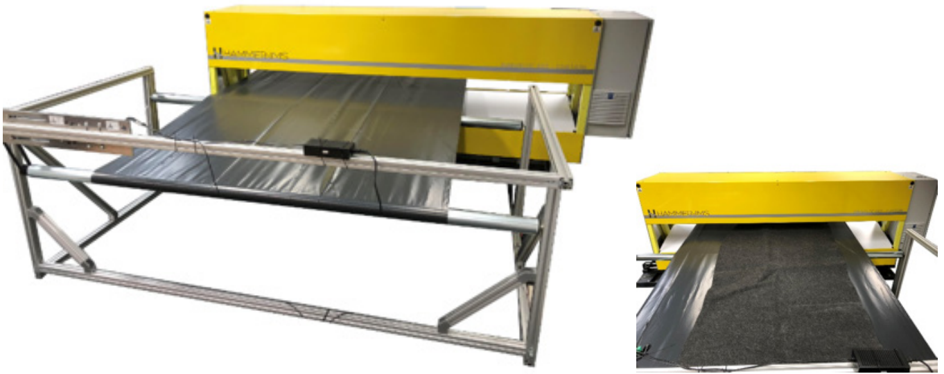
Figure: Left: A 200 micron PVC film is used as a carrier material to convey a non-woven material through the scanner, making a laboratory-device scanner system setup. Right: When applying a nonwoven material on the film, 100 % quality control is enabled in an offline setting.
