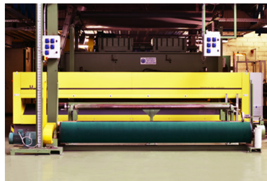
Figure: The Marveloc 602-CURTAIN scanning frame containing 4 M-Ray sensors, scanning basis-weight of nonwoven converting lines in real time.
