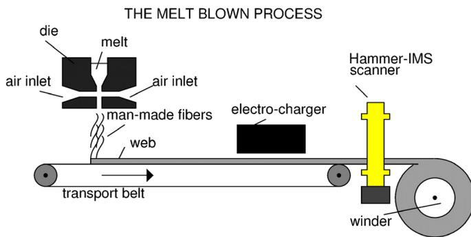
The meltblown process excels in its simplicity and conversion time, yet it is the most performant process to make permeable materials. A die contains a heated polymer melt, which is blown-out by two controlled air blowers on opposite sides on the die, creating a cloud of man-made fibers with a fineness that can go down to a few 100 nanometers. The cloud is sucked against a collector media, which is either a belt or a roller. Electro-charging further
