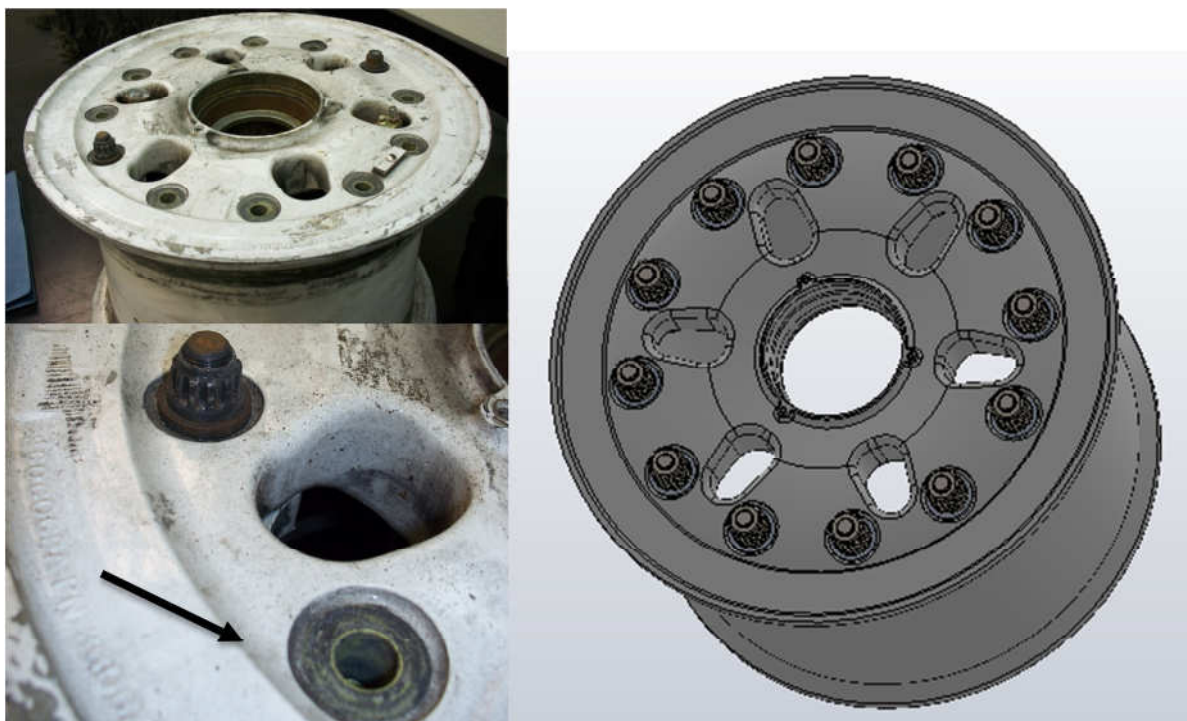
Figure 1 Forged Al wheel with corresponding computational model – arrow shows corroded area
