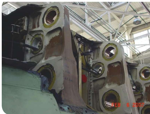
FIGURE 1 Corrosion in F-18 wing-fuselage attach bulkheads. 8
