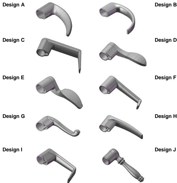
**Figure 1: simplified CAD configuration of 10 door handle designs**
