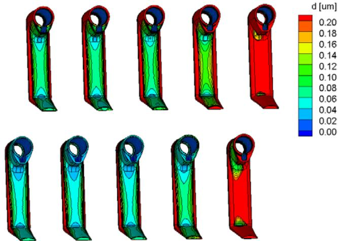
Figure 7: Cr layer thickness distribution over lower parts on rack, Case 1
