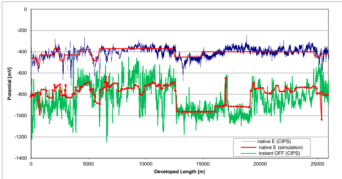
Figure 10: Comparison between simulated potentials and CIPS survey data
