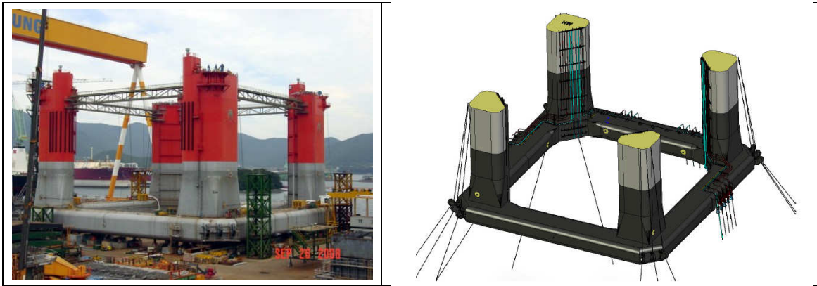
Figure 9: CAD model of Opti-Ex™ (submerged parts) with initial ICCP system
