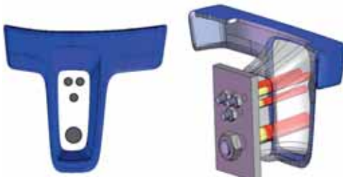
Abb. 7: Simulation mit 4 Innenanoden Figure 7: Simulation with four auxiliary anodes
