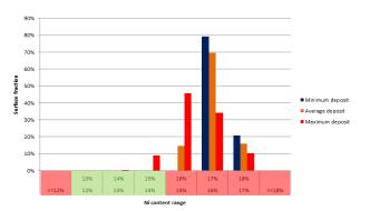
To better illustrate the usefulness of the bar charts, the bath type used in this example has an operating window from 12 to 18% in nickel and thus a large portion of the parts shows excessive nickel content. The nickel excess can be immediately identified in the bar chart.
