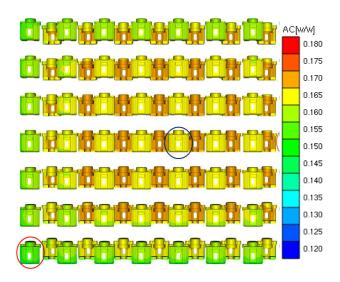
The same color plot is presented for the nickel content distribution. For this electrolyte, nickel content decreases with increasing current density, thus the parts around the edge of the rack show a lower nickel content than those in the centre of the rack.
