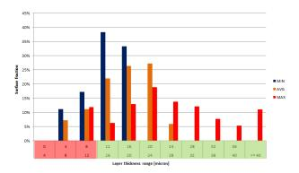
In the bar chart above the layer thickness is segmented in layer thickness ranges, in this case every 4 microns, and the corresponding surface fraction that falls within this interval is presented. The first blue bar indicates that around 11% of the surface (of the minimum deposit part) is between 4 and 8 microns in layer thickness.
