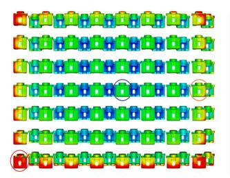
The color plot clearly depicts the increased deposit thickness for the parts that are located at the edges of the rack, yet somewhat limited on the right hand side, where the 2nd rack is situated (not shown here). Although the 2nd rack is present the space between then is still large enough to create a noticeable edge effect at these positions too.
