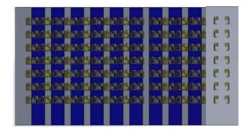
Simulation results include current density and layer thickness color plots for the entire rack and additional statistical information for 3 selected parts. To better illustrate the spread in results across the rack, the parts across the rack that receive the lowest (= part A), highest (= part B) and average deposit weight (= part C) are identified.
