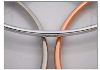
Cu/Ni/Cr plated parts after Neolink pretreatment.
