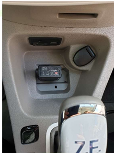
Figure 62 – OBD2 reader installed.
