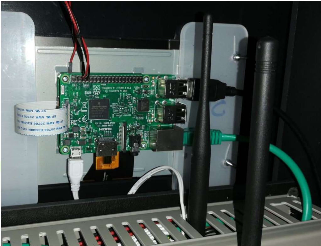
Figure 70 – Raspberry Pi 3, installed in EMOT EVSE, used for WiseEVP laboratory tests.
