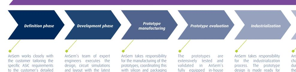
The chip architecture and the circuit topologies are studied and defined. Testability, reliability and qualification requirements are discussed. A final ASIC specification is agreed with the customer.
