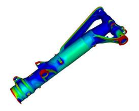
By addressing each problem zone at a time via iterative simulations, a complete package of auxiliary anodes, current robbers and insulating shields is developed. Different rectifiers act on separate zones to achieve enhanced control over the current density distribution. This finally leads to deposit thickness that is within specifications over 95 to 100 % of the surface area to be plated.
