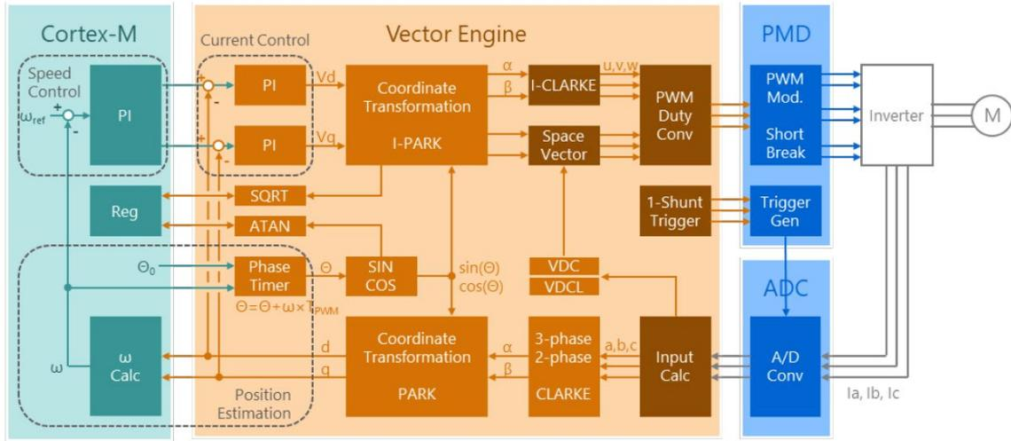
*Block diagram of a FOC based implementation for driving BLDC motors*
