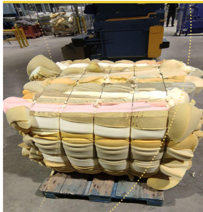
Polyurethane foam ball for recycling: it comes from the press in which cut foam blocks are compacted © Envie 2E Lorraine
