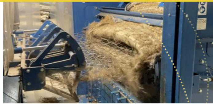
Separation of the textile materials from the metal spring by tearing off the spring: the textile previously pre-cut on the front of the mattress is held by seams while a clamp pulls the spring. © Envie 2E Lorraine
